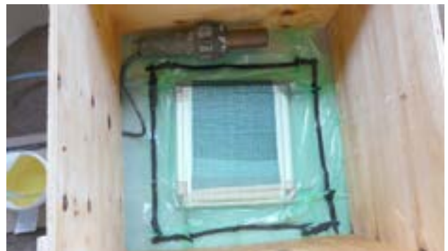
Figure 3.2.23. Infusion of the cross ply.
