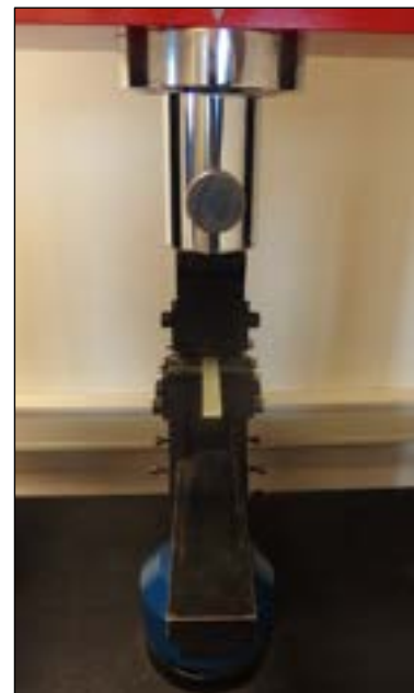
Fig. 6 centered and aligned specimen
