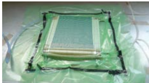
Figure 3.2.16. check the vacuum bag for leaks.
