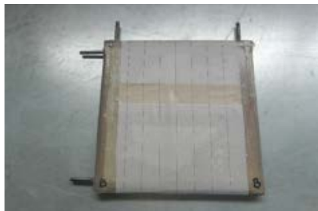
Figure 2.2.3, Applied and taped peel ply. Taped side marked with
