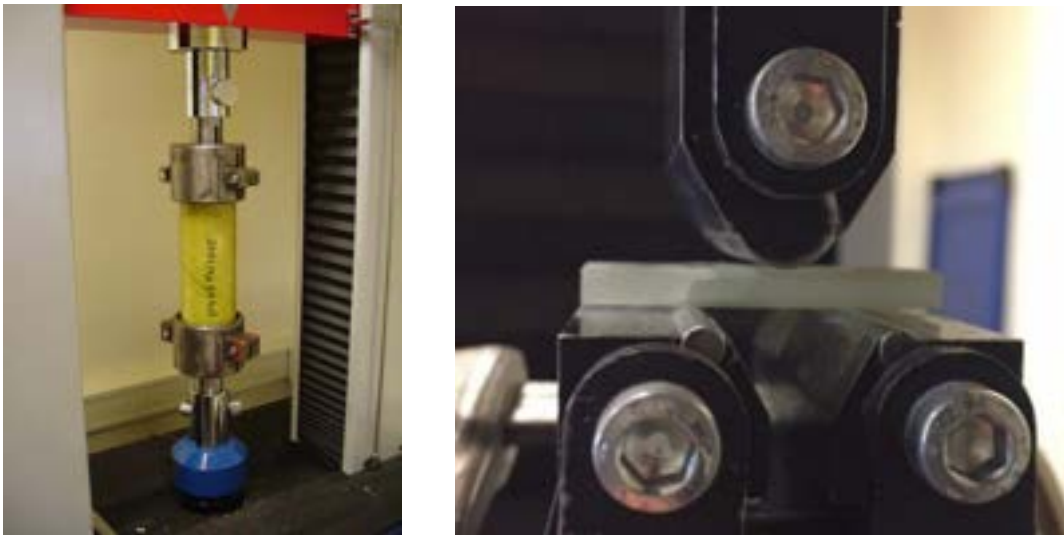
Figure 6. Left, Axial Tensile Test (ATS) on pipe. Right, Inter Laminar Shear Strength (ILSS) test.
