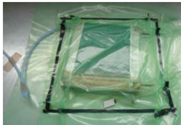
Figure 3.2.12. tape clamp at the injection tube (inlet).
