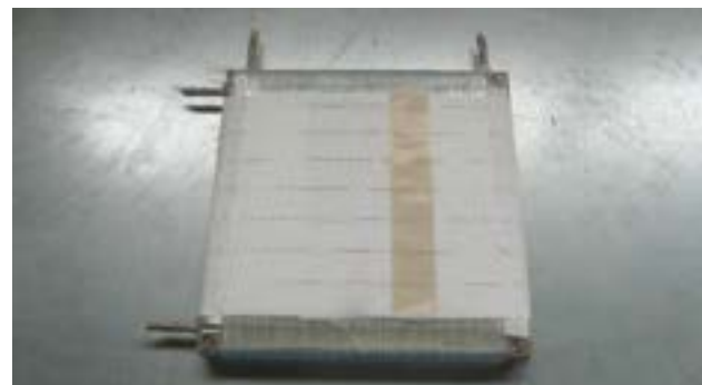
Figure 3.2.2. peel ply taped at the bottom side and covered threaded ends.
