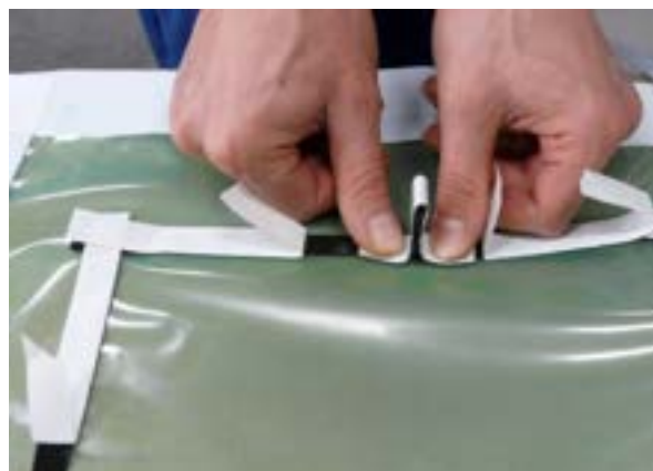
Figure 3.2.9. tape loops at the corner of the square.
