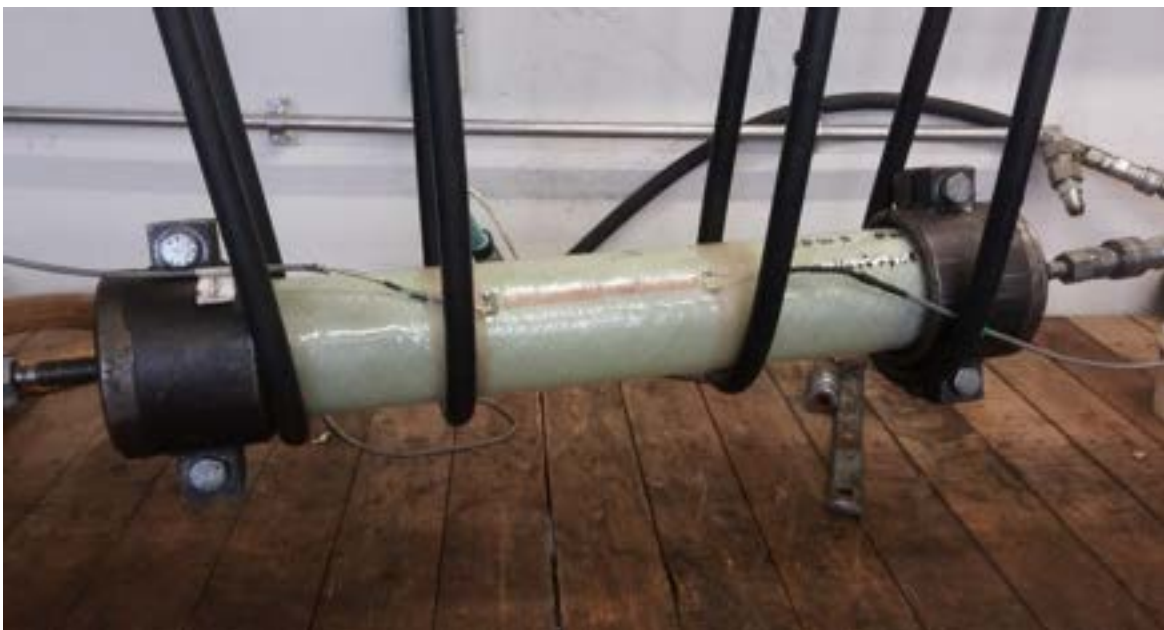
Figure 5. Ultimate Elastic Wall Stress (UEWS) setup
