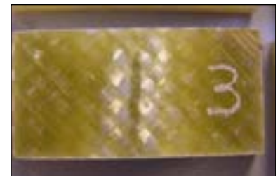
Fig. 8 Flexure by compression
