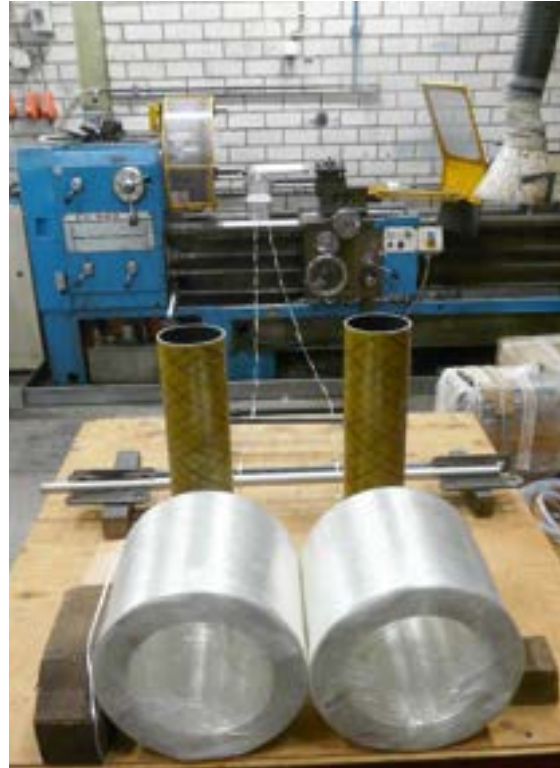
Figure 2.3.1. overview dry winding setup.
