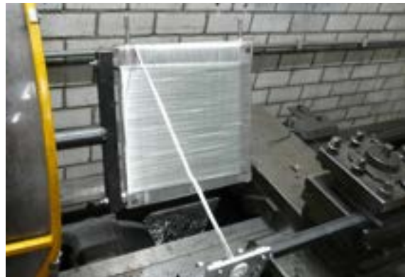
Figure 2.6.4. rotated and turned mould after second layer.
