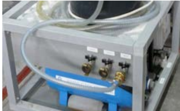
Figure 3.2.14. vacuum hose connected to the tap of the vacuum pump.
