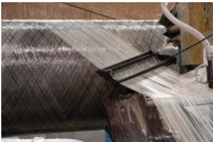
Figure 2. Production of GRE pipes via winding
