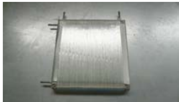
Figure 2.6.5. completed cross ply.
