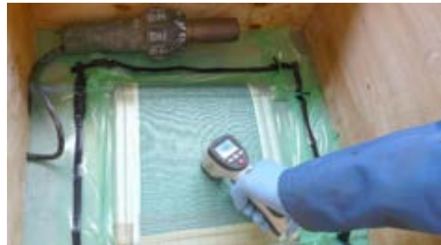
Figure 3.2.22. check the temperature at the top of the vacuum bag.
