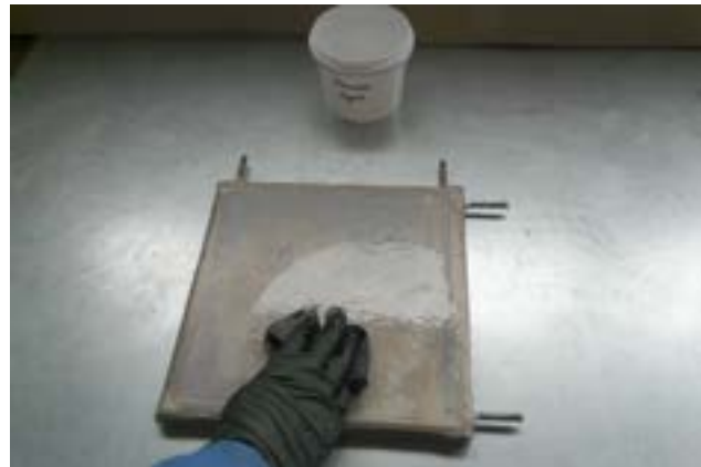
Figure 2.2.2, Polish the applied release agent.
