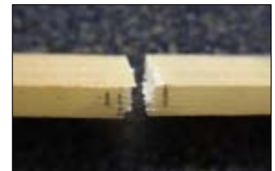
Fig. 9 Breaking by tension
