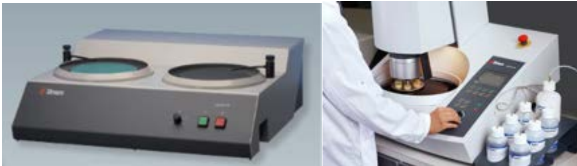
Figure 27. An illustration of a Struers hand polishing system for larger grain sizes. (Right) A photograph of a Struers polishing system for smaller grain sizes using diamond powder as a polishing medium.
