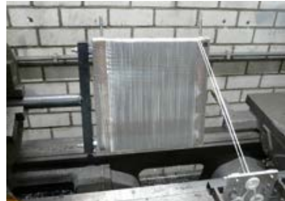
Figure 2.6.2. first layer in 0° direction.
