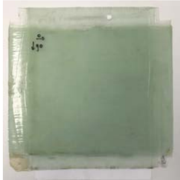
Figure 3.2.24. removed peel ply and written layer direction.
