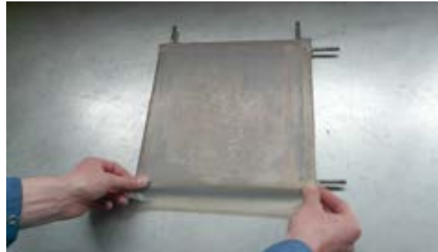
Figure 2.2.1, Teflon at corners and edges of the mould.
