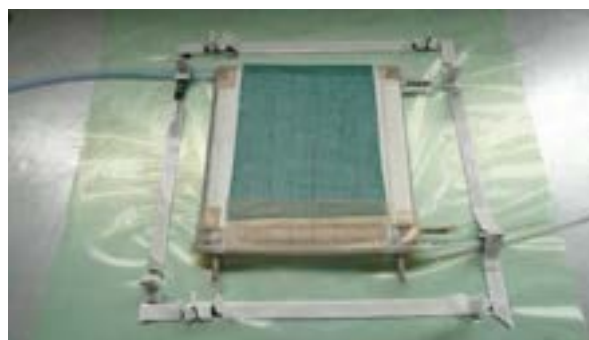
Figure 3.2.10. inlet and outlet tubes at the corner of the square.
